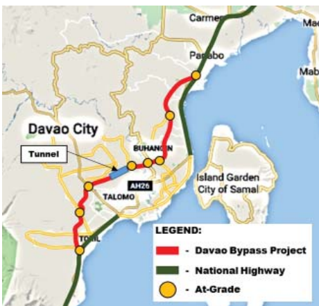
The planned 44.6-kilometer Davao City Bypass Road, which aims to mitigate congestion in the city. Image courtesy of DPWH
